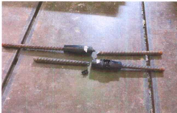
Figure 1 Tensile failure of deformed bar.
